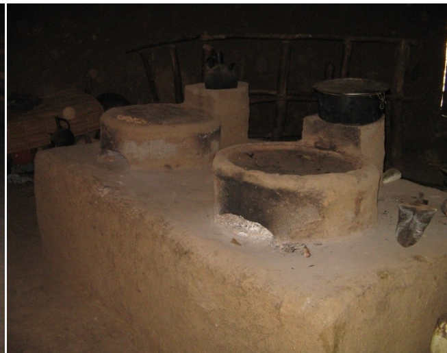
Photo 3.2: Twin Mirt stoves (one for Injera & the other for Kocho) in use in a rural household, near Hosaena town
