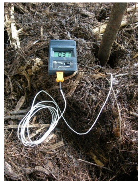
Illustration 6: Temperature measurement with type K thermocouple
